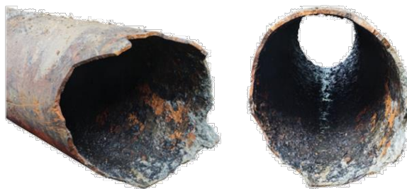
700 mm cast iron water pipe broken by water hammer
