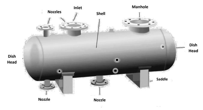
**Pressure vessels** are critical components used in various industries, including oil and gas, chemical manufacturing and power generation. Their primary function is to contain gases or liquids at high pressure, so their integrity is essential for safety and operational efficiency.
